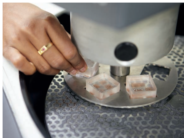
Resined block samples on a polishing disc being prepared for analysis.
