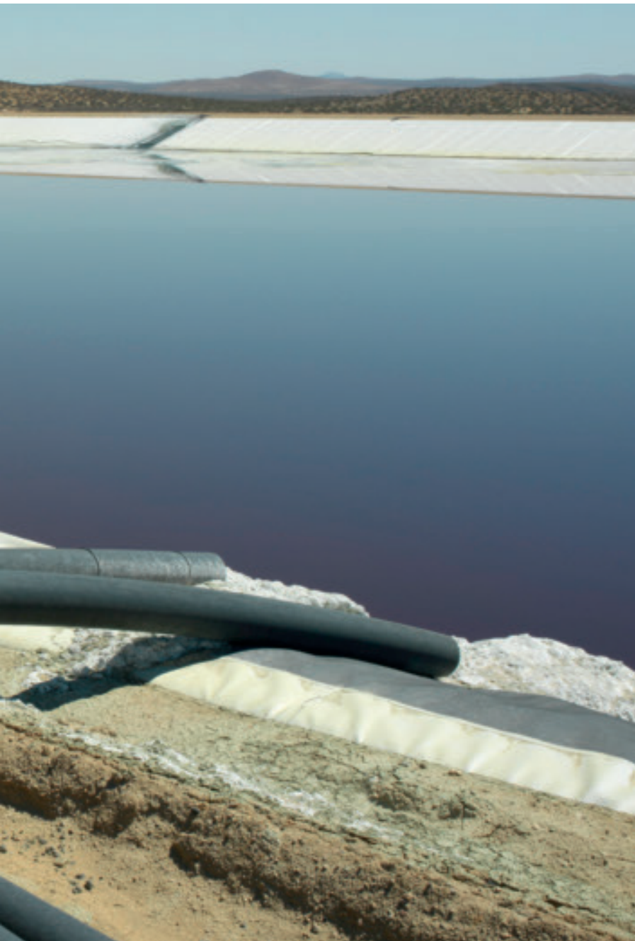
Borate rich liquids from the production process captured in ponds and left to evaporate are now being re-mined (below) for further processing.
