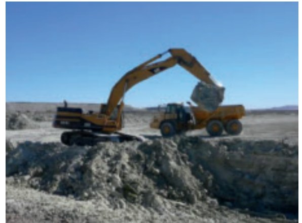
Borate rich liquids from the production process captured in ponds and left to evaporate are now being re-mined (below) for further processing.
