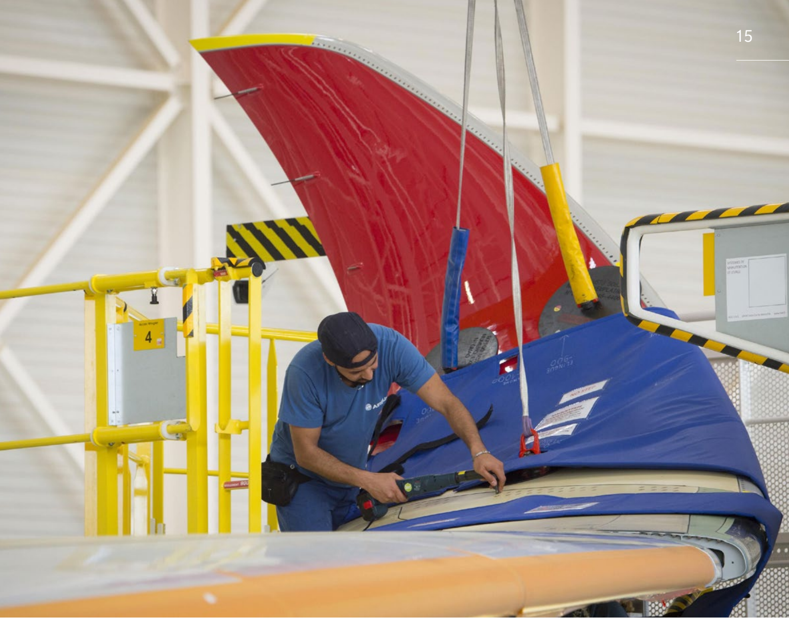
Assembly of the first Air Mauritius A350 XWB with its state-of-the-art aerodynamic morphing wing at Airbus' Final Assembly Line in Toulouse, France. The aircraft is 25 per cent more fuel efficient than the previous generation aircraft. Source: Airbus
