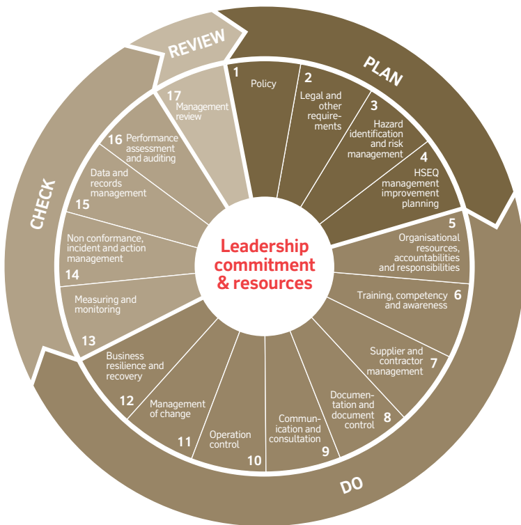
[Figure 1 – The Rio Tinto HSEQ management system standard's continual improvement cycle showing the four phases and 17 Elements.]
